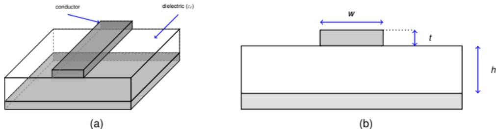
Figure 8 : Microstrip transmission line
