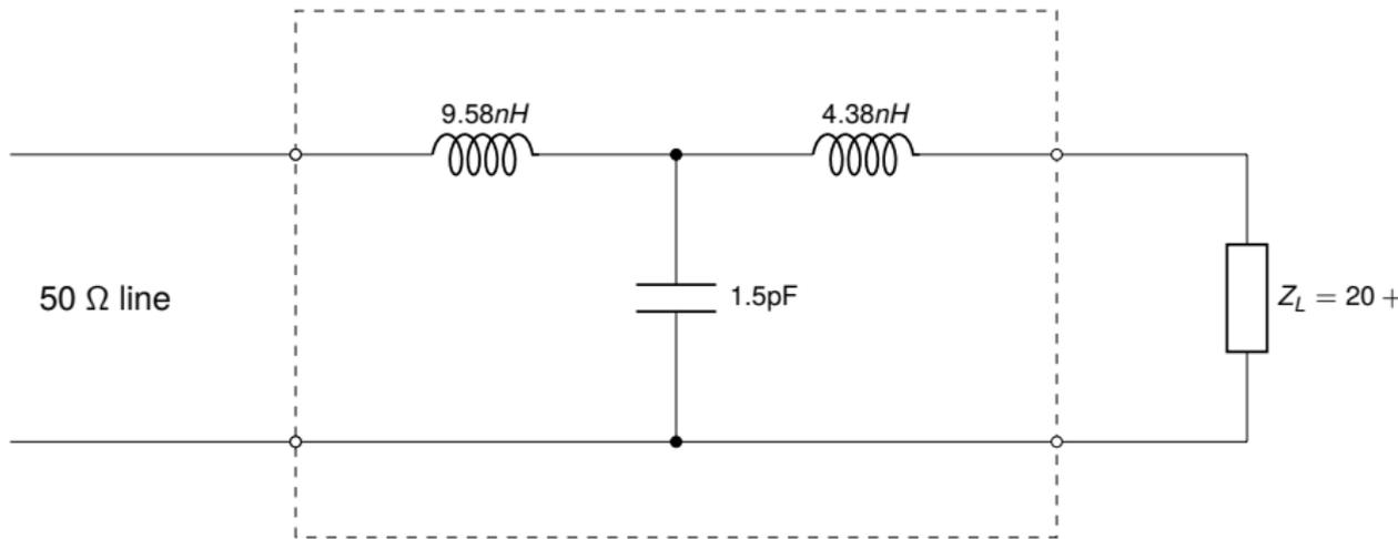
Figure 15 : T-section matching network example - final configuration
