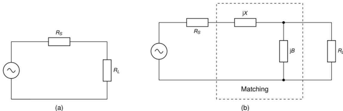
Figure 3 : Matching arbitrary  $R_L$  and  $R_S$
