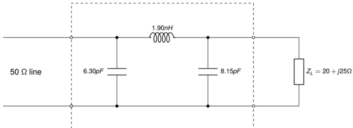
Figure 12 :  $\pi$ -section matching network example - final configuration
