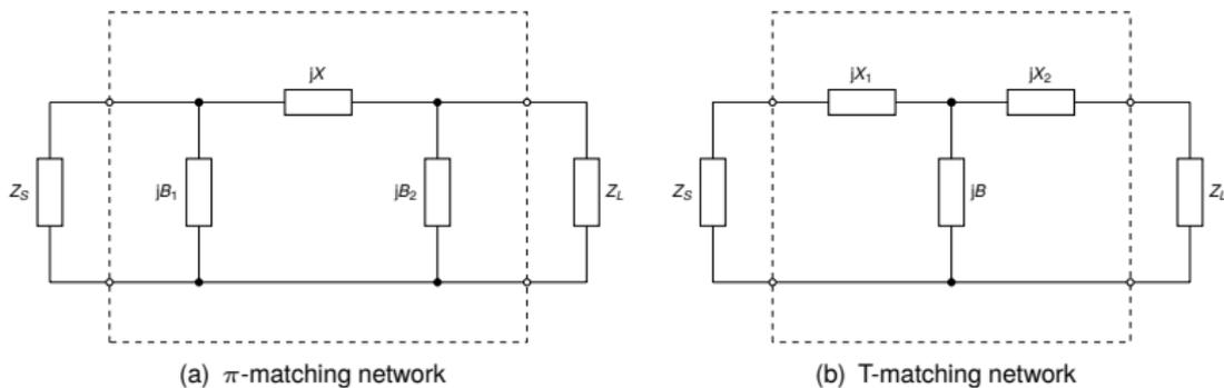
Figure 6 : Three element matching networks
