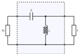
Type 1a can only match capacitive loads lying outside unit admittance circle or inductive loads lying inside unit resistance circle
