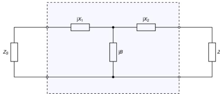
The T-Section can be considered as consisting of a type 2 L-section and type 1 L-section in cascade as shown below, where  $B = B_1 + B_2$  :
