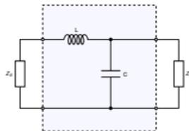
Type 1b can only match inductive loads lying outside unit admittance circle or capacitive loads lying inside unit resistance circle
