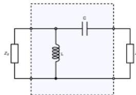
Type 2b can only match inductive loads lying outside unit resistance circle or capacitive loads lying inside unit admittance circle
