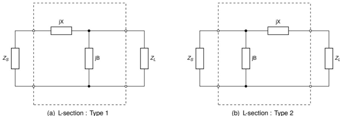
Figure 4 : Generalised L-section matching networks
