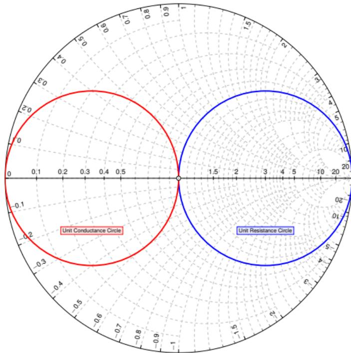
Figure 5 : Unit conductance and resistance circles
