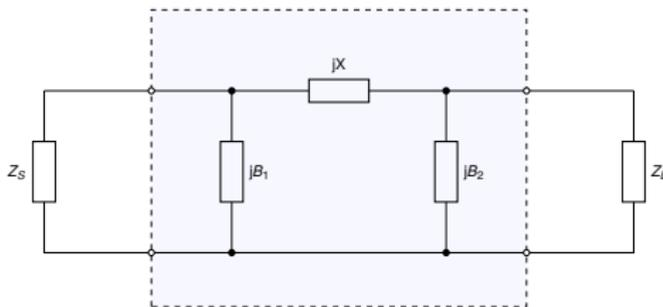
Figure 7 :  $\pi$ -section matching network
