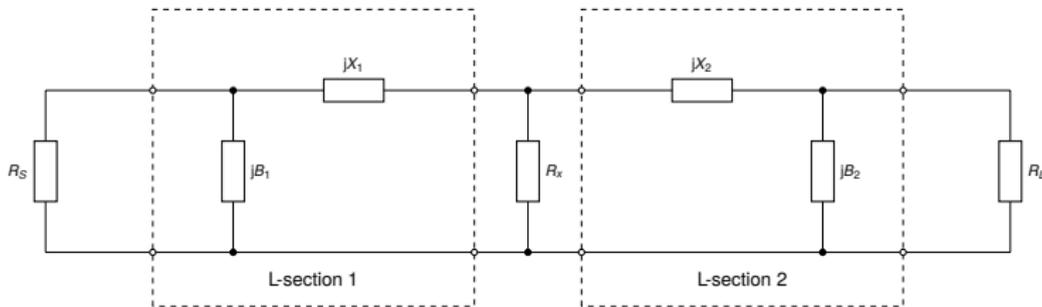
Figure 9 :  $\pi$ -section matching network as a cascade of two L networks
