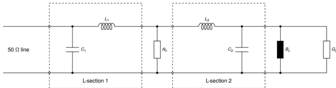
Figure 11 :  $\pi$ -section matching network example
