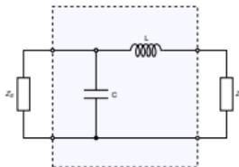
Type 2a can only match capacitive loads lying outside unit resistance circle or inductive loads lying inside unit admittance circle
