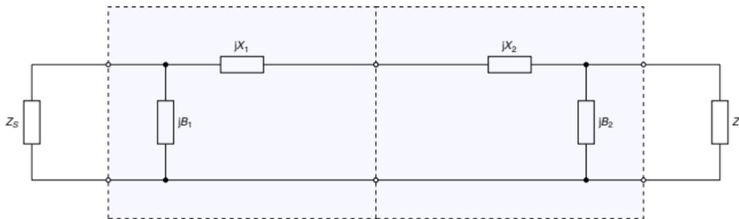
Figure 8 :  $\pi$ -section matching network
