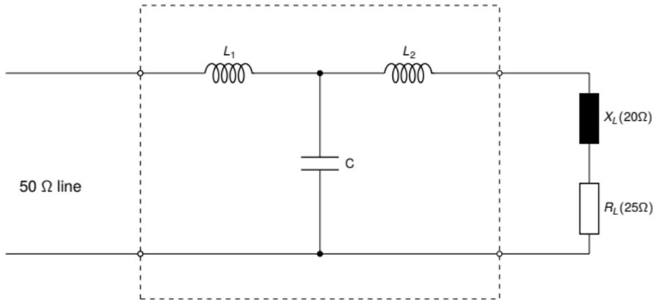
Figure 14 : T-section matching network example
