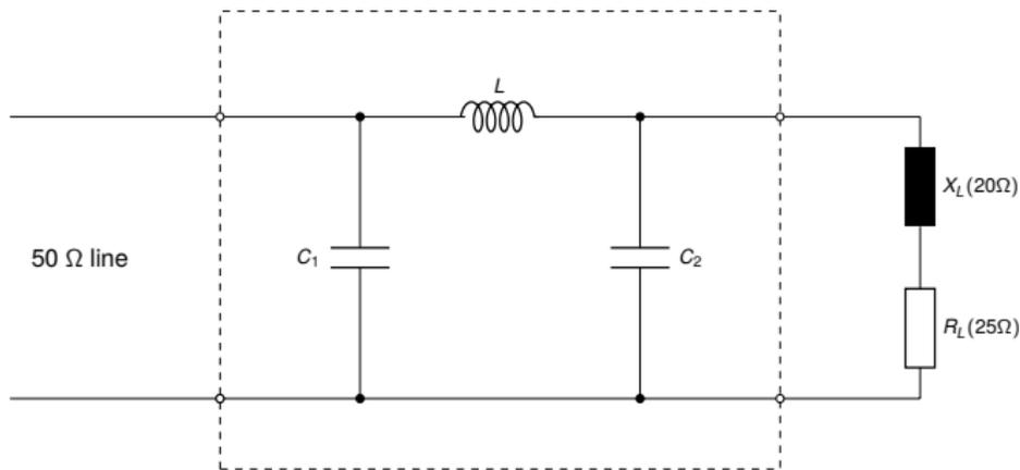
Figure 10 :  $\pi$ -section matching network example
